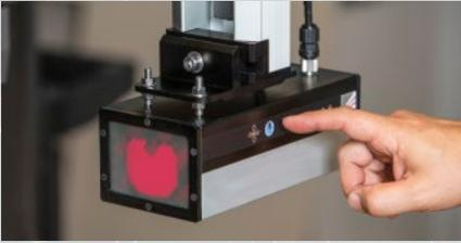
The Sentinel Plus camera receiver features automatic tool alignment that eliminates the need for precise manual adjustment and reduces tool set-up time. After tool change simply press the TOOL ALIGN button on the receiver. The receiver scans the punch to locate the tool tip then automatically adjusts the protection zone.
